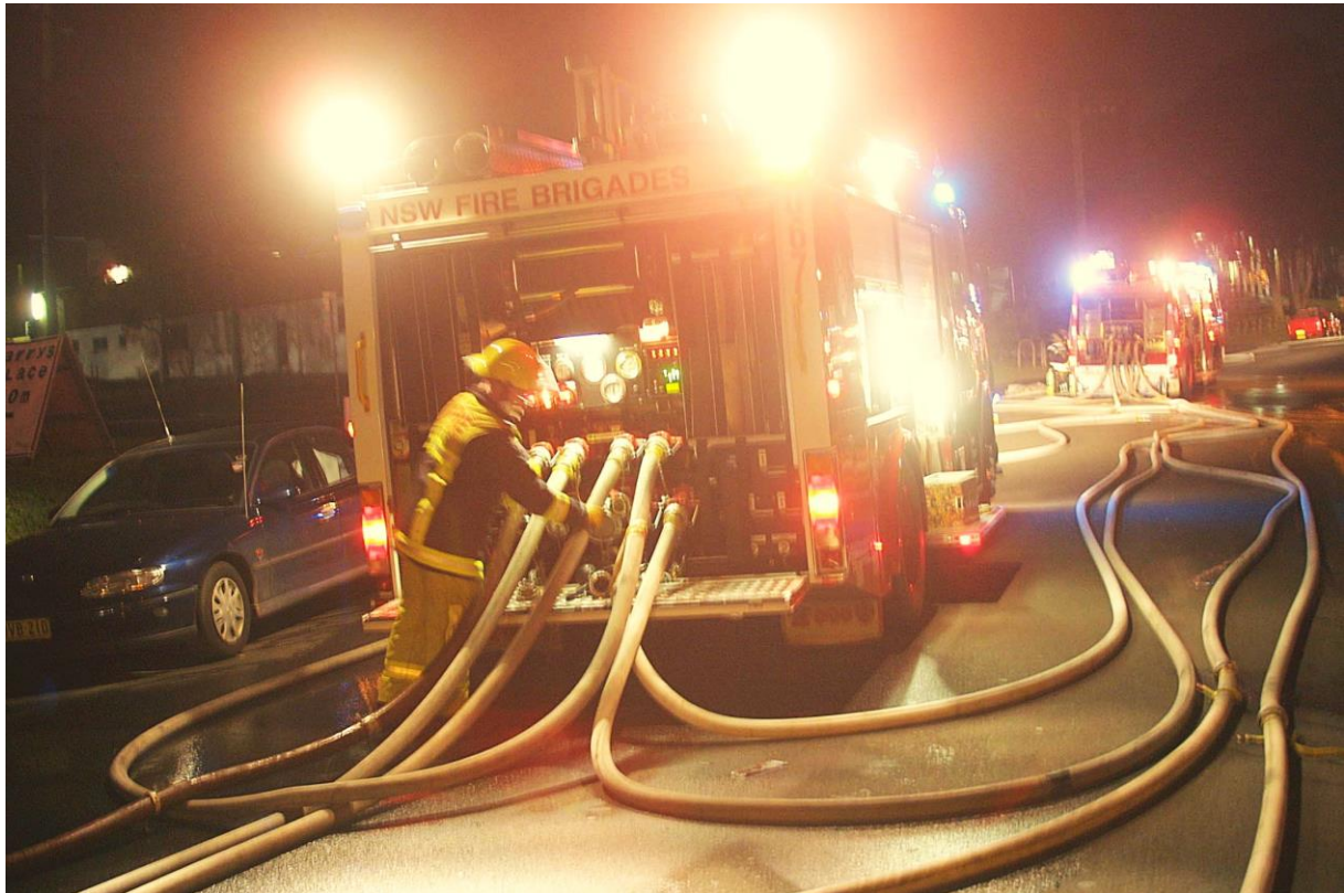
Establishment of an effective water supply was absolutely critical to containing the fire and achieving fire control. Firefighters established multiple water relays. Top: Pumper 27 supplies water to Ladder Platform 27. Lower: Pumpers 67 and 57 relay water to the fireground. Successful relay pumping is a critical requirement at major structure fires. Firefighting can only be effective if there are adequate water supplies.
