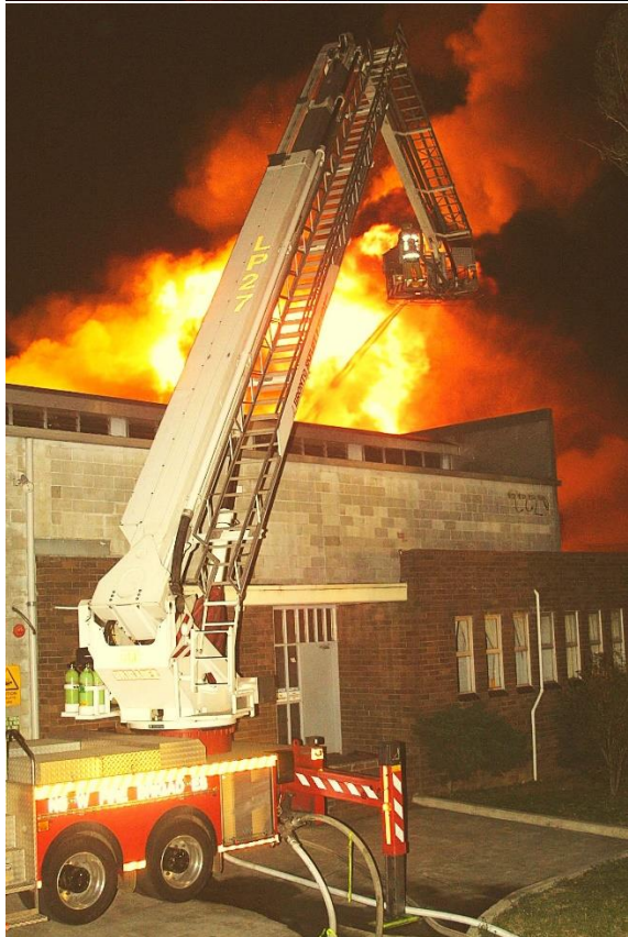
Exposures on all sides of the factory came under significant threat. Ladder Platform 27 directs a protective steam along the eastern wall of Exposure B. Firefighters have gained entry into Exposure D, where fire is beginning to enter the factory through a collapse wall.
