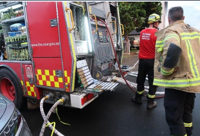
First arriving Hazmat Pumper 77 became the key focal point of operations. Pump operator Chris Joseph is managing water, pumping operations and water supply to fire attack lines, as well as Main B.A. Control (consisting of two Stage I B.A. Control Boards), radio communications base and staging point for the on-deck crews (RP102 Firefighters Bruce Annabel and Felicity ralphs). Out of site, a rehabilitation area and decontamination area have also been established. This work was just as important as putting water on the fire.
