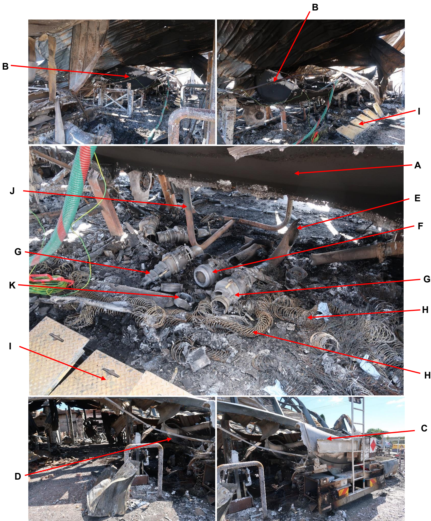
The tanker following the fire: A Tanker shell, B Tanker shell bulkhead (forward), C Tanker shell bulkhead (rear), D Internal compartment wall, E Pipe from compartment to outlet (x 6), F outlet valves fitted with standard camlocks (x 6), G Outlet adaptor (x 6), H Static lines fitted to tanker unloading hoses (x 6), I Underground tank fill point covers (x 6), J Unloading valve assembly under-tank collision protection bar, K hose coupling.
