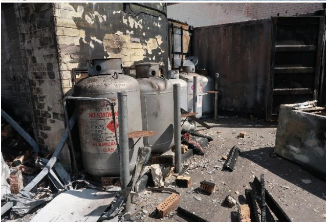
Seven 210 kg LPG cylinders were located at the front of the service station retail building and a storage shipping container. The impact of intense heat from the tanker fire resulted in boiling liquid expanding vapour explosions (BLEVEs) occurring to two of the cylinders. Firefighters directed cooling streams onto the remaining cylinders, preventing further BLEVEs from occurring.
