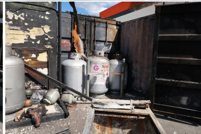
Seven 210 kg LPG cylinders were located at the front of the service station retail building and a storage shipping container. The impact of intense heat from the tanker fire resulted in boiling liquid expanding vapour explosions (BLEVEs) occurring to two of the cylinders. Firefighters directed cooling streams onto the remaining cylinders, preventing further BLEVEs from occurring.
