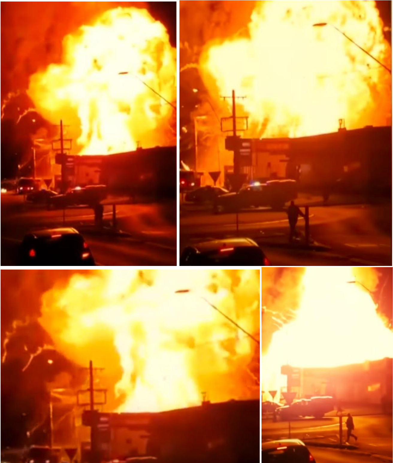
Taken by members of the public these photographs show boiling liquid expanding vapour explosions (BLEVEs) occurring involving 210 kg LPG cylinders. These photographs were taken from a distance of approximately 250 metres from the service station and are indicative of the size and intensity of the explosions.
