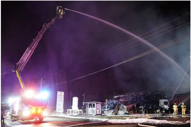
Firefighters place CAFS Aerial Pumper 47 in operation as a water tower. The presence of high-voltage overhead powerlines and initial water supply shortages restricted aerial appliance operations. Middle left – Firefighters cool the 8,000 litre LPG bulk storage tank.
