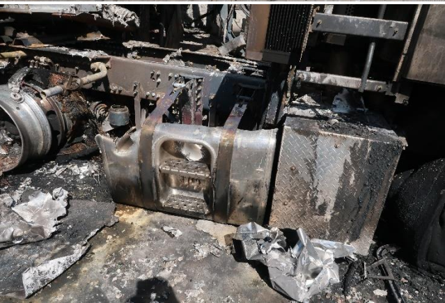
Most of the aluminium components melted. Steel rims are visible and only the steel belts of the tyres remain on most of the wheels of the prime mover.
