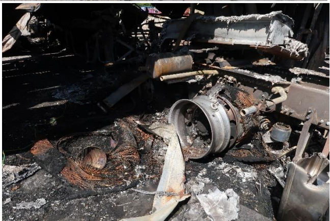
Most of the aluminium components melted. Steel rims are visible and only the steel belts of the tyres remain on most of the wheels of the prime mover.
